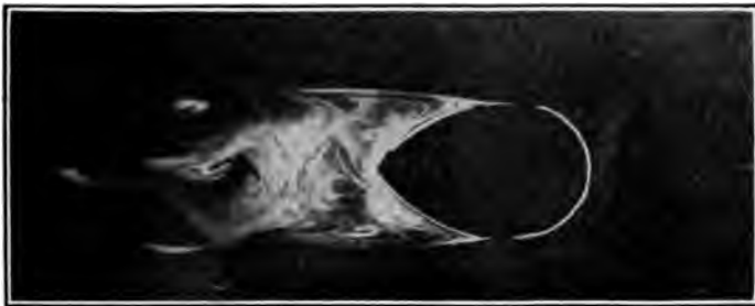
FIG. 17. FLOW FOR A SHORT STRUT.
